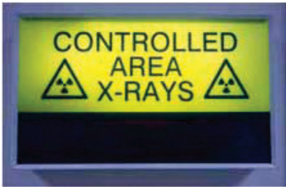
Figure 16: External flashing radiation warning sign during CT x-ray exposure
