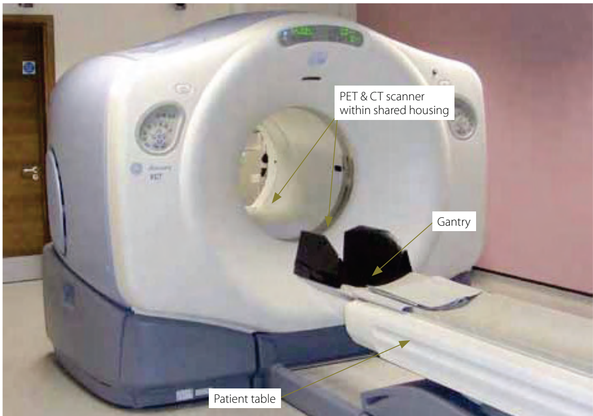
Figure 2: A typical PET-CT scanner
